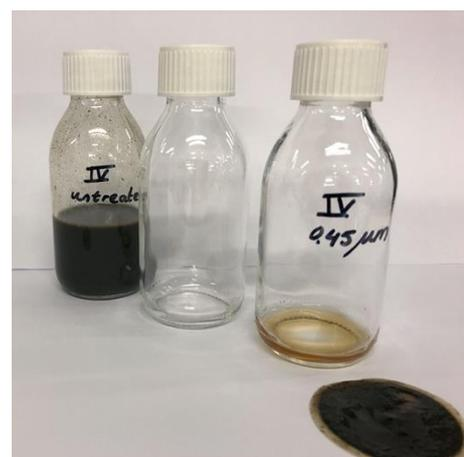
Figure 15: Fraction VI: Thin digestate: untreated and 0.45 µm SDI permeate and the fouling layer on the membrane used for SDI determination.
