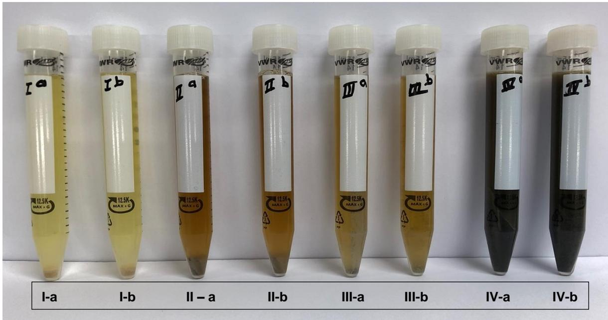
Figure 13: Separation between solid and liquid phase after centrifugation (3 minutes @ 6500 rpm) for all obtained samples.
