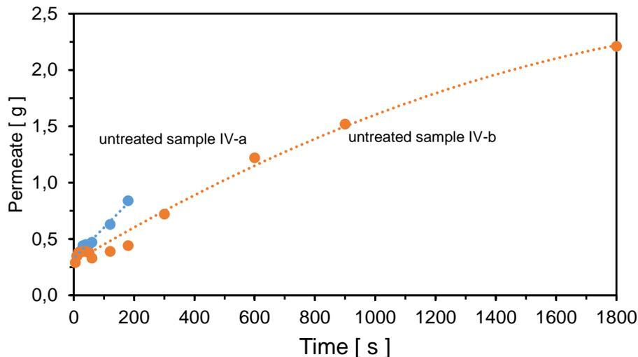
Figure 17: SDI filtration curves of thin digestate (IV).
