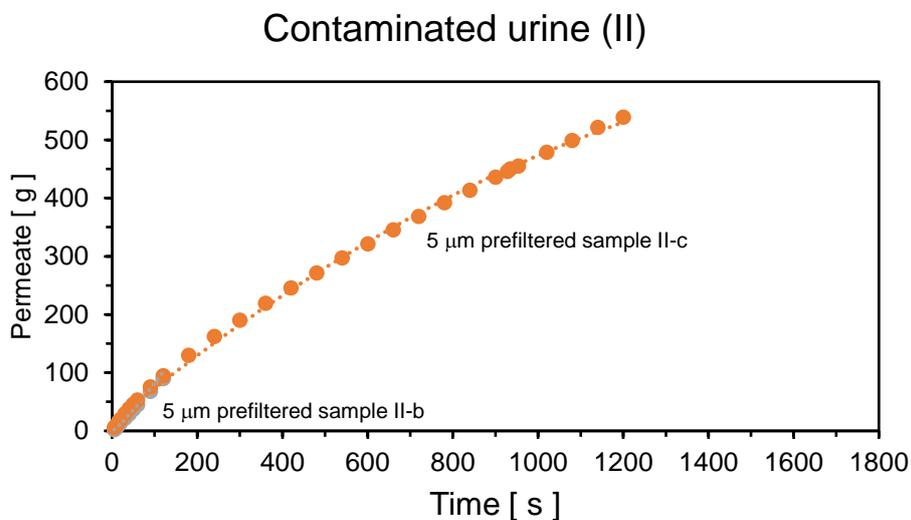
Figure 21: SDI filtration curve of contaminated urine (II).
