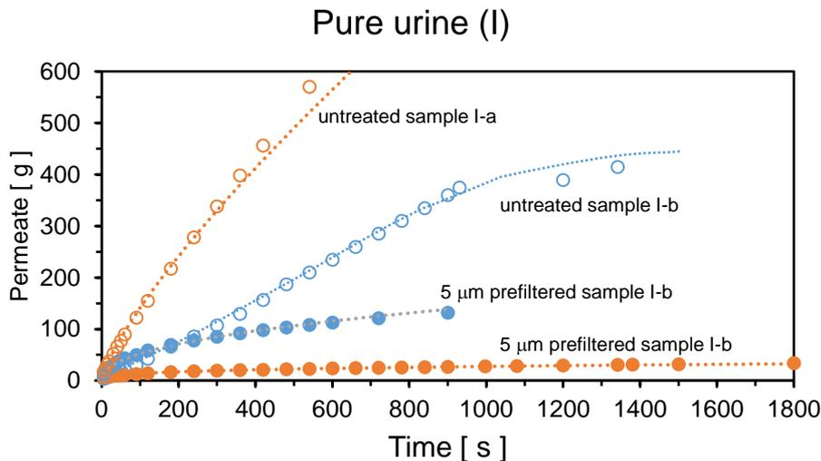
Figure 21: SDI filtration curve of pure urine (I).
