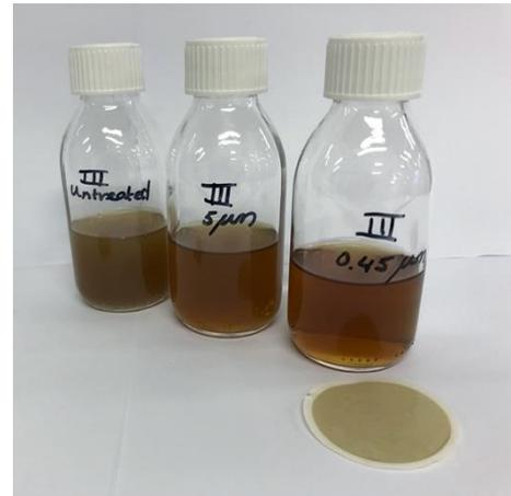
Figure 18: Fraction III: Thin manure: untreated, 0.5  $\mu m$  prefiltered and 0.45  $\mu m$  SDI permeate and the fouling layer on the membrane used for SDI determination.
