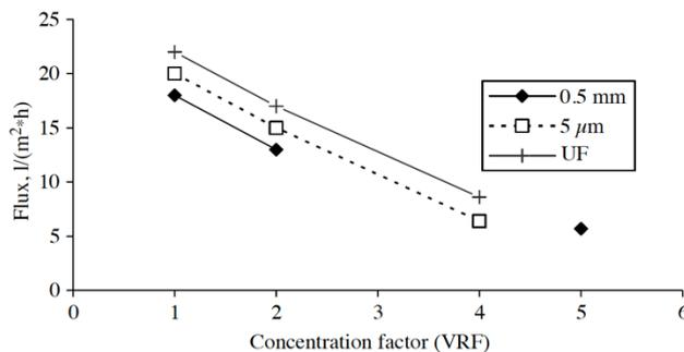
Figure 9: Flux as a function of the volume reduction factor (VRF) and type of pre-treatment for urine RO filtration [14].
