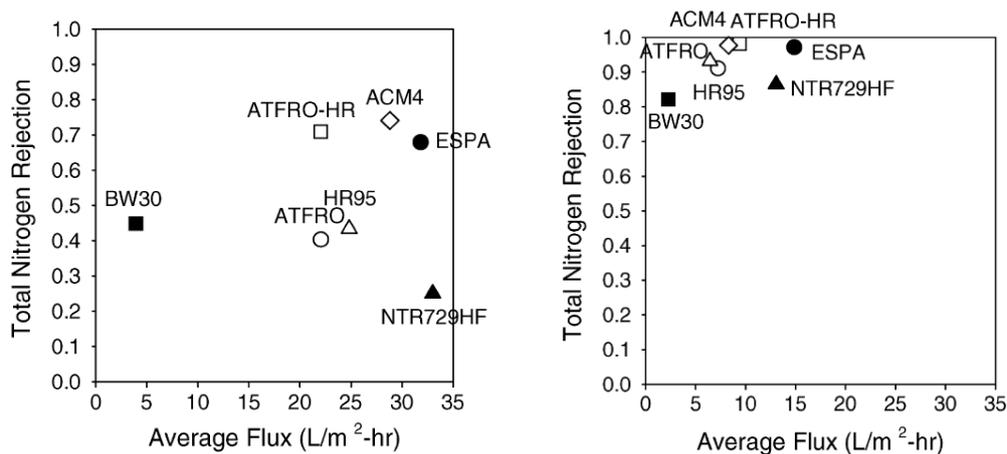
Figure 3: Total nitrogen rejection by different RO membranes with synthetic wastewater containing A) urea and creatine as nitrogen source (left) and wastewater B containing  $\text{NH}_4^+$  as nitrogen source (right). Operating conditions: 800 kPa, stirring speed: 400 rpm, salt concentration: 0.02 M, 60% recovery [7].
