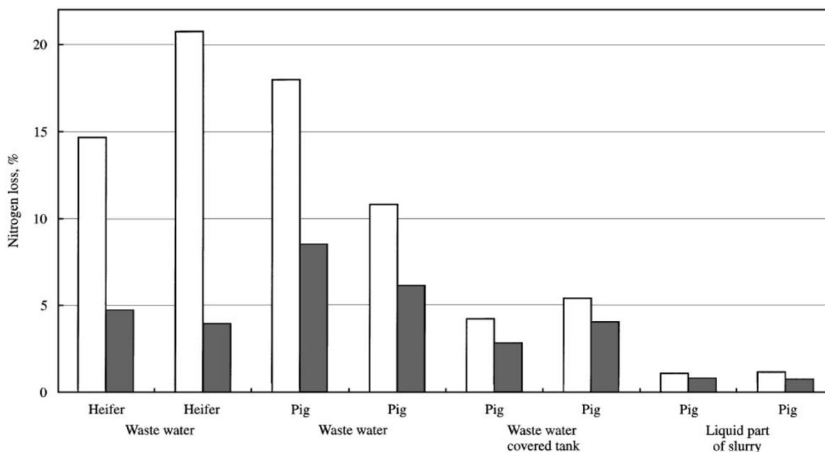
Figure 8: Total loss of nitrogen (white columns) and nitrogen loss to permeate (gray columns) for different feeds from Farm A, B and C [11].
