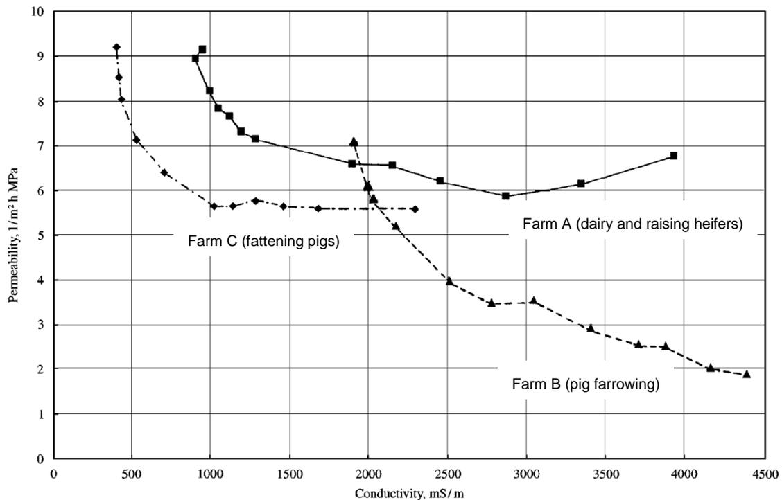
Figure 6: Temperature normalized permeability as a function of estimated conductivity for wastewater from farm A, B and C [11]. For comparison: fluxes obtained at reference Farm III (Manure) are in the order of 1-2 l/m<sup>2</sup> h bar.
