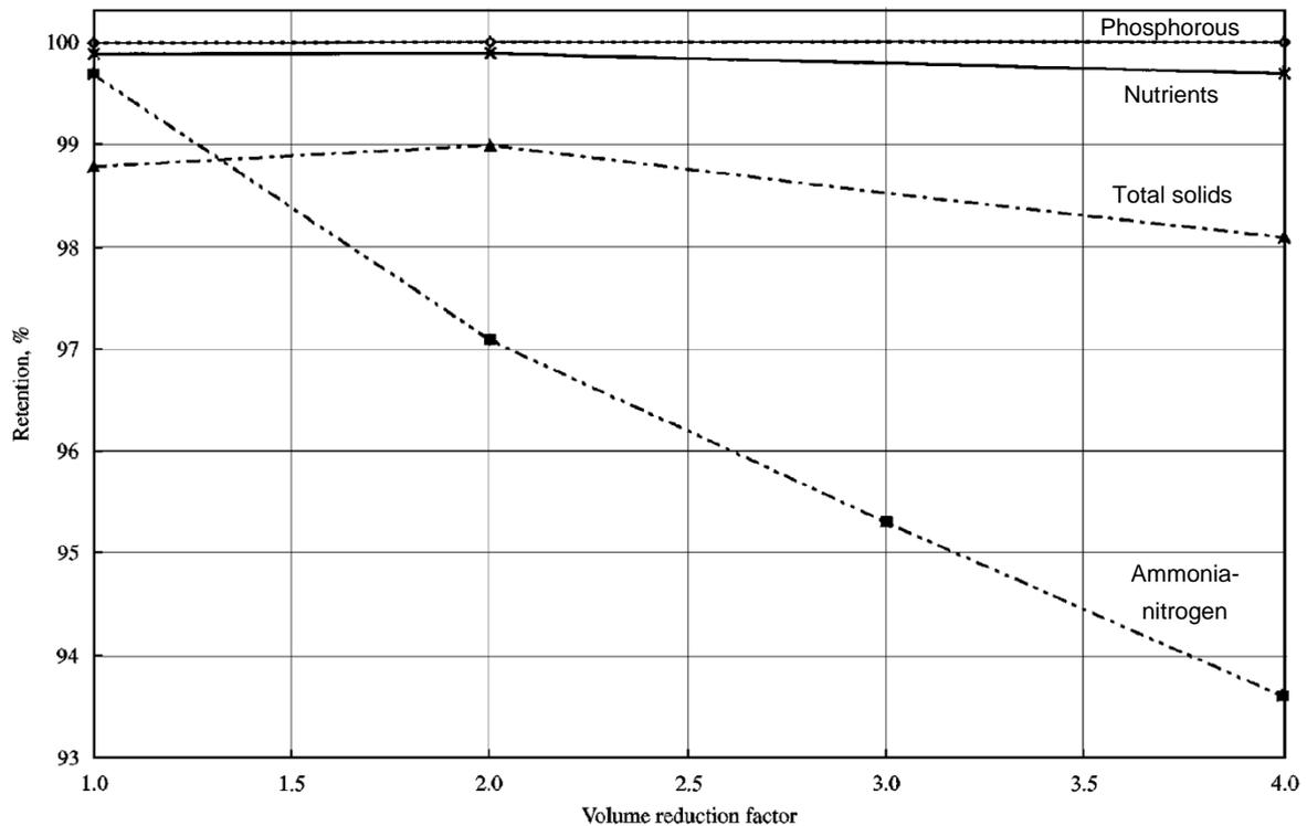
Figure 7: Retention of ammonia-nitrogen, nutrients (determined via COD - chemical oxygen demand), phosphorous and total solids [11].
