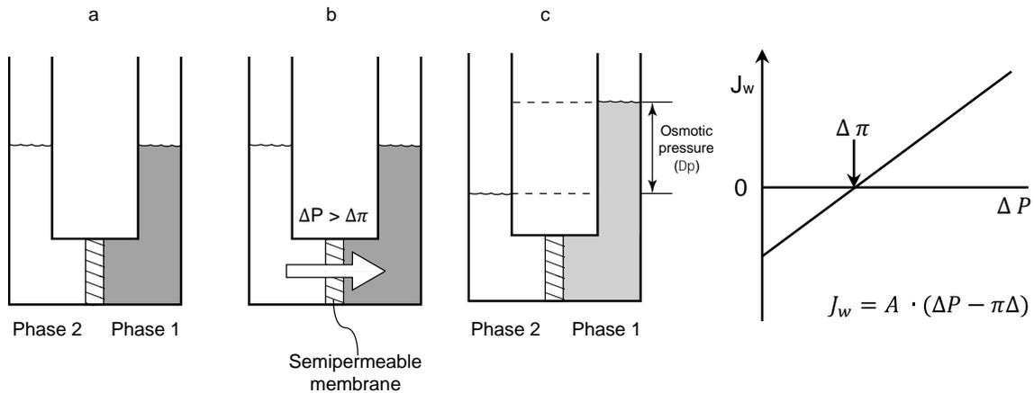
Figure 1: Schematic drawing of osmosis and the water flux ( $J_w$ ) as a function of the applied mechanical pressure [2].
