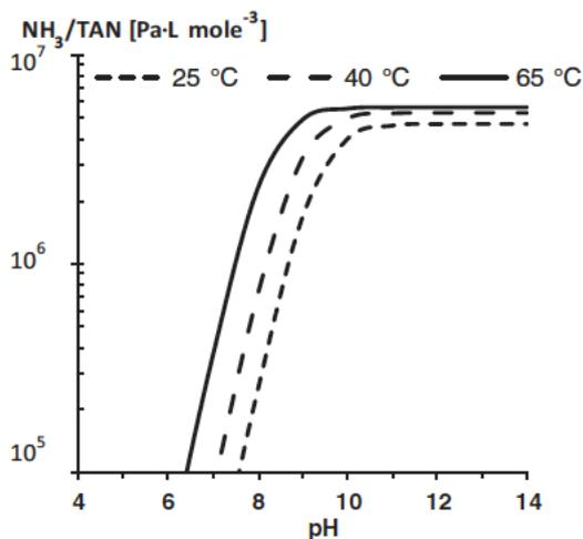
Figure 2: Influence of pH and temperature on the partial pressure of  $\text{NH}_3$  [4].
