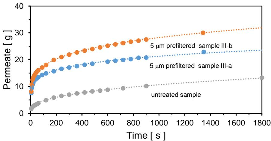
Figure 19: SDI filtration curves of thin manure (III).
