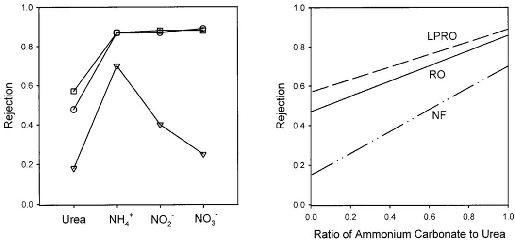
Figure 5: Left: effect of nitrogen form on experimentally measured rejection of urea, NH<sub>4</sub><sup>+</sup> (ammonium carbonate), NO<sub>2</sub><sup>-</sup> (sodium nitrite), and NO<sub>3</sub><sup>-</sup> (sodium nitrate). Experimental conditions: 800 kPa, stirring speed: 400 rpm, feed concentration: 250 mg N/liter. Right: theoretical estimate of the dependence of rejection on the ratio of ammonium carbonate to urea at similar conditions [8].
