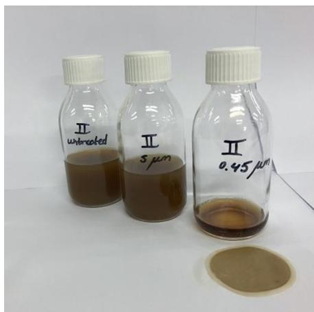
Figure 20: Fraction II: Contaminated urine: untreated, 0.5 μm prefiltered and 0.45 μm SDI permeate and the fouling layer on the membrane used for SDI determination.
