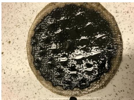
Figure 16: Sample IV digestate: due to the highly viscous, high solids solution, severe fouling occurred and only a few ml of permeate could be collected. Image shows precipitation of 25 ml filtrate on a type 2 paper band filter (Farm III).
