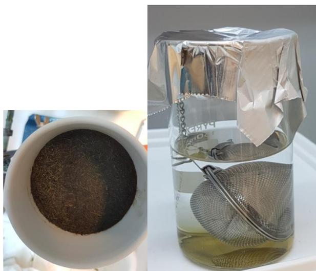
Solid-Liquid extraction was repeated three times, using ultrasonic bath 30 °C for 15 min. The three collected fractions were merged and evaporated until 2-3 ml volume and then filtered through a Lichrolut vial equipped with glass frit. The filter was then flushed with Methanol/Ethyl acetate 50/50, % v/v to obtain approximately 8-10 ml total of filtrate.
