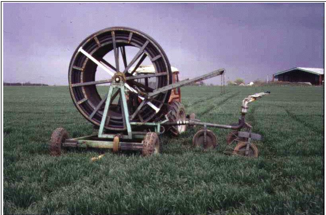
Figure 2.32: Example of a raingun
