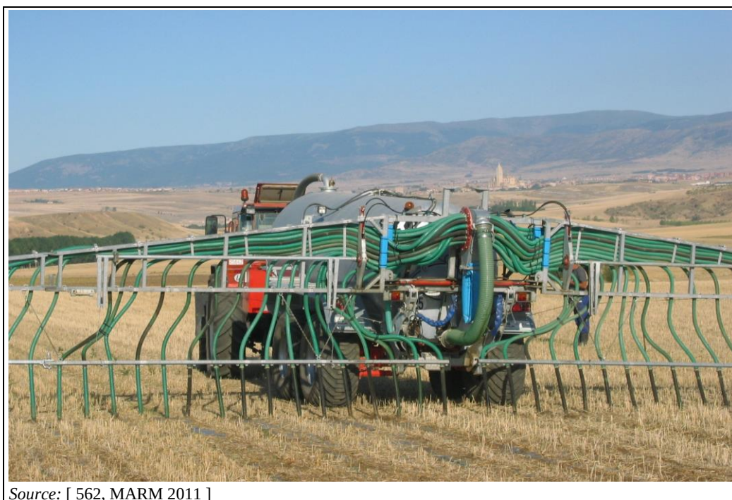
Figure 2.37: Example of a band spreader fitted with rotary distributor to improve lateral distribution
