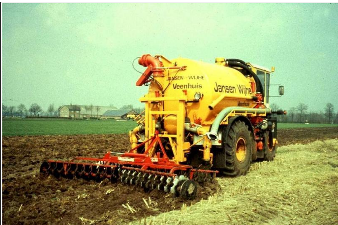
Figure 4.101: Incorporation equipment combined with a big tanker
