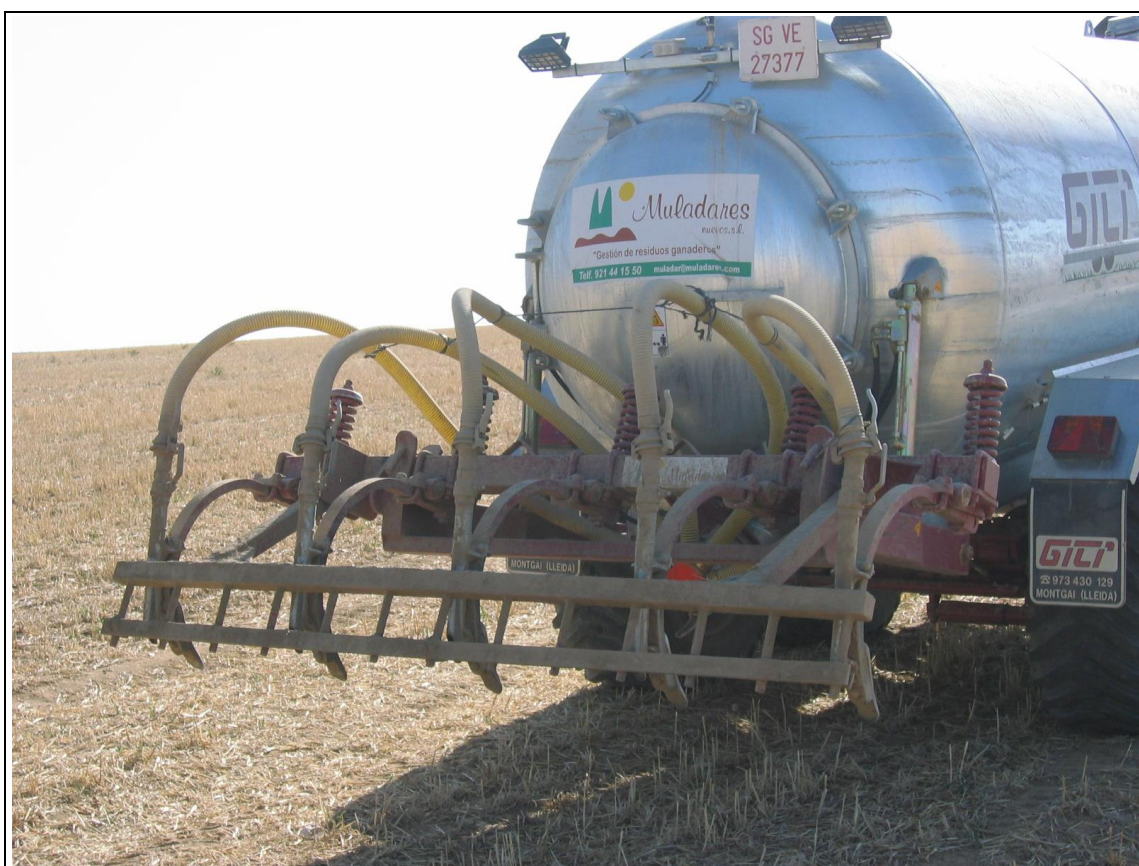
Figure 2.38: Example of an open slot injector
