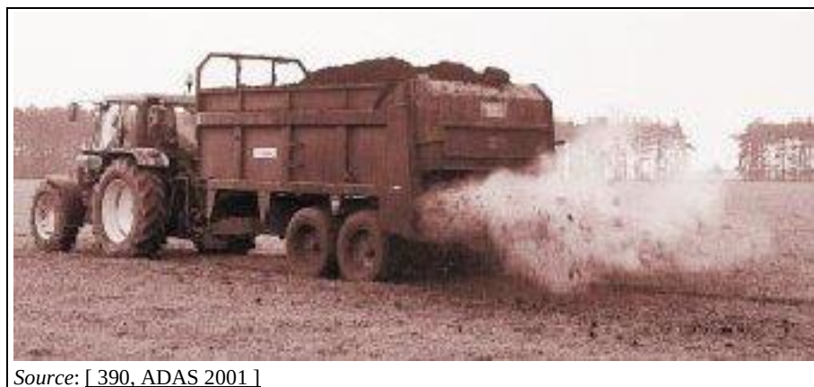
Figure 2.40: Example of a rear discharge spreader
