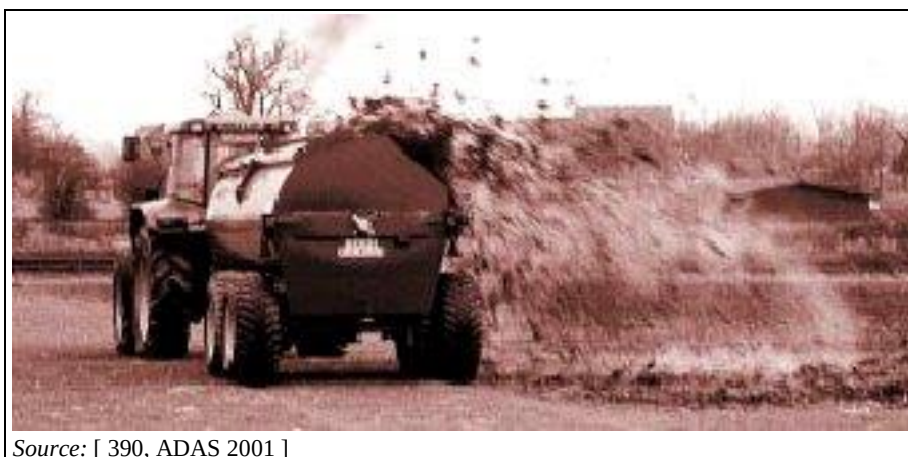
Figure 2.39: Example of a rotaspreeder
