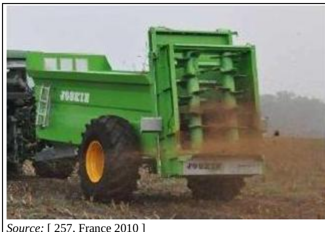
Figure 2.42: Vertical drum manure spreader
