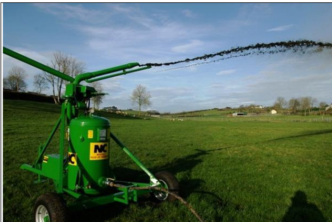
Figure 4.96: Pulse-jet irrigator in operation
