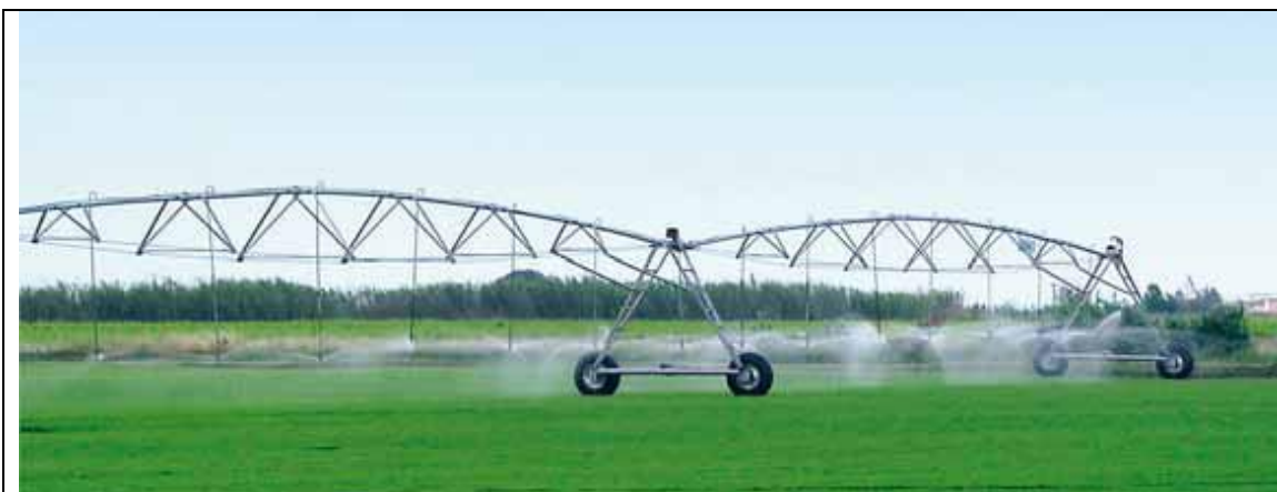
Figure 4.95: Irrigation boom fitted with hanging nozzles to spray the water-slurry mixture close to the soil surface
